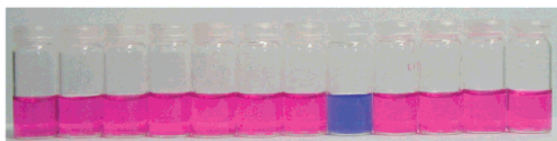
Figure 1. Color changes on solution of L^1 (see text, [L^1] = 5 \times 10^{-5} mol \text{dm}^{-3} ) in water:acetonitrile, 1:1 v/v, in the presence of certain anions at pH 9 and further addition of 30 \mu\text{L} of \text{H}_2\text{SO}_4 (30%). From left to right; no anion, fluoride, chloride, bromide, iodide, acetate, benzoate, sulfide, phosphate, sulfate, nitrate, and cyanide.
